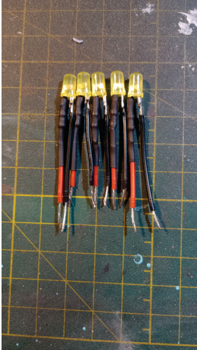
5 Yellow LEDs with resistors, positive and negative leads soldered on. Heat shrink tubing is also applied.
